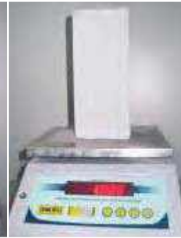
Flyocrete A.A.C. Block cut to brick size. Found 1 kg
